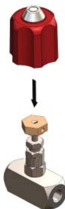
5. Push the lock assembly onto the adaptor
